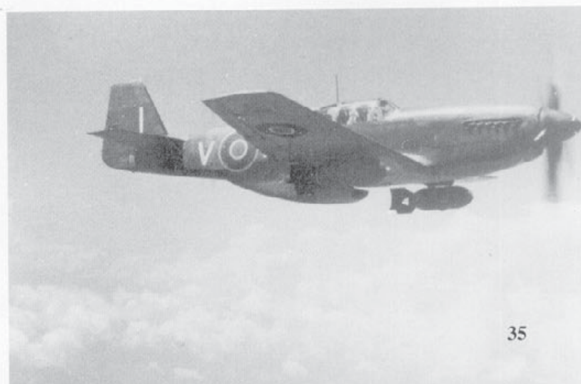
A Royal Air Force Mustang III fighter bomber from No 250 Sudan Squadron, enroute to targets in Italy during 1944. The fighter-bomber Mustangs could carry a pair of 1,000 pound bombs under the wings. (via Jeff Ethell)
