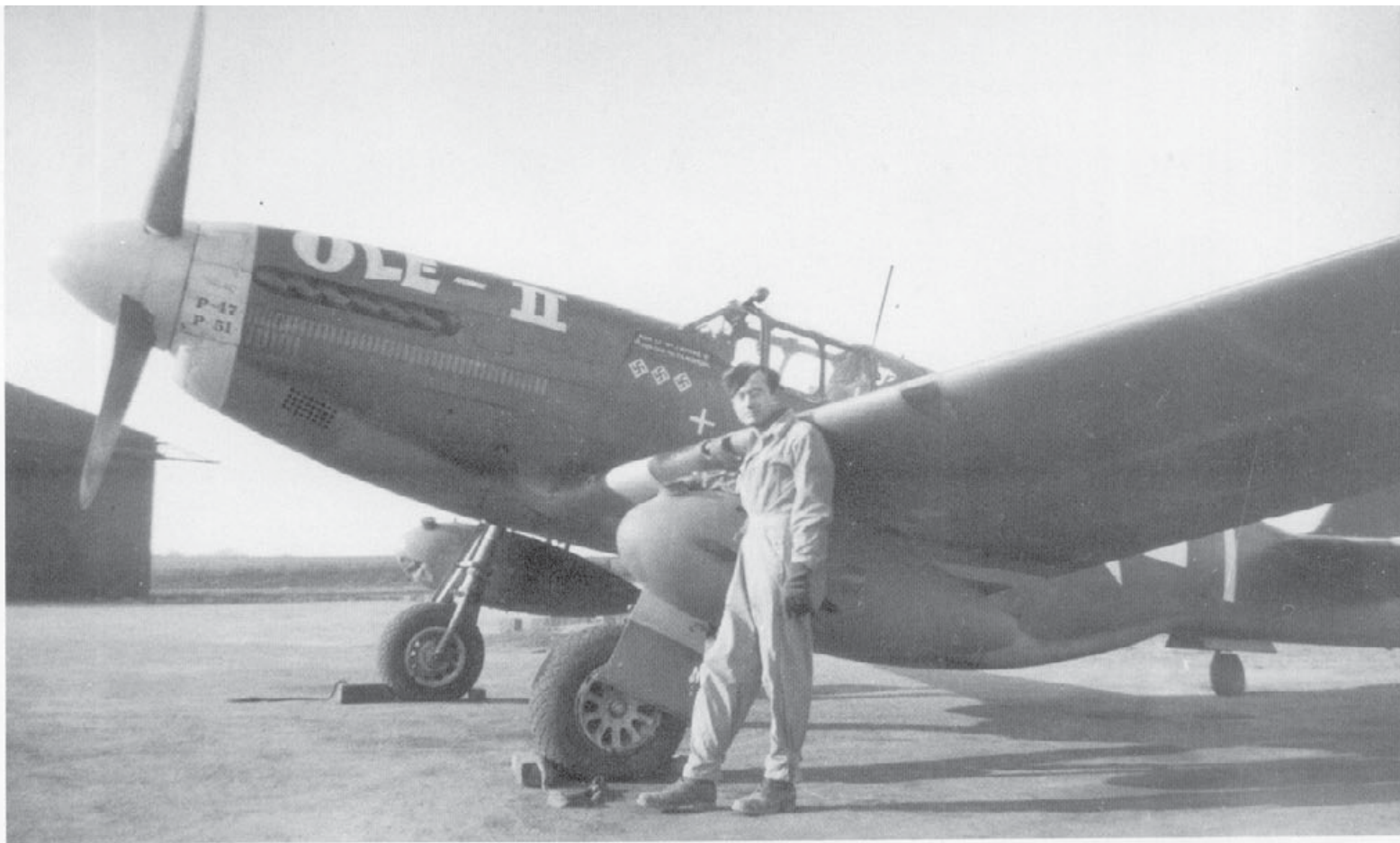
Lieutenant William Hovde flew Ole-II , a P-51B of the 358th Fighter Squadron at Steeple Morden. The scoreboard shows forty-eight P-47 missions before conversion to the P-51B in March of 1944. Hovde's P-51B has a pair of Spitfire rear view mirrors mounted on top the windscreen. (Keith Melville)
