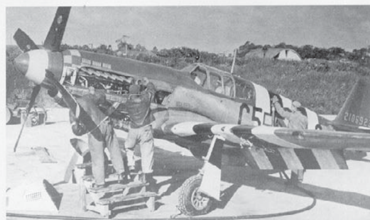
Two mechanics in the 364th Fighter Squadron work on the big Merlin in this P-51B at Leiston, as a third refuels the Mustang for another mission on D-Day, 6 June 1944. (Keith melville)
