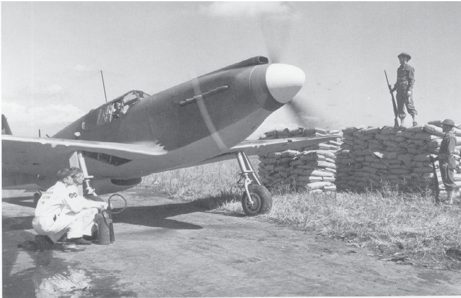
A staged posing of a new production RAF Mustang I at Mines Field (now the site of LA International) during 1942. The Mustang I was delivered in the standard RAF camouflage of Dark Earth and Dark Green, with Sky undersurfaces. The lengthened carburetor scoop was an identification feature of all production Allison-engined Mustangs. (NAA)
