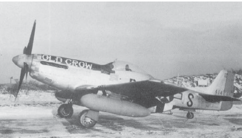
The last of Captain Clarence Anderson's Old Crow's sits on the snow-covered 363rd Fighter Squadron ramp at Yoxford with eighteen victory markings on the fuselage under the windscreen. The aircraft also carried two 110 gallon pressed paper drop tanks. (Merle Olmsted)
