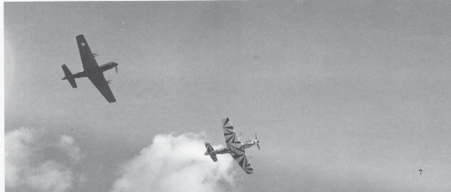
A pair of P-51s fly side-by-side to show off the underside pattern of Captain Paul Hexter's disruptive paint scheme. The upper surfaces were painted standard Olive Drab. The "dazzle" scheme was meant to disrupt an enemy gunners aiming point, but was never adopted for operational use. (USAAF)
