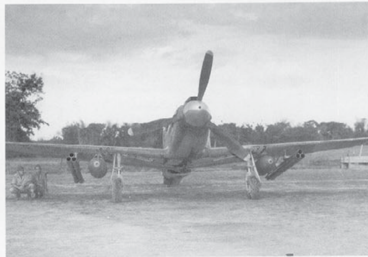
A 1st ACG P-51A sits on the Dinjan ramp armed with a pair of 500 pound bombs and six underwing 5 inch Bazooka rocket launchers during August of 1944. (USAAF)
