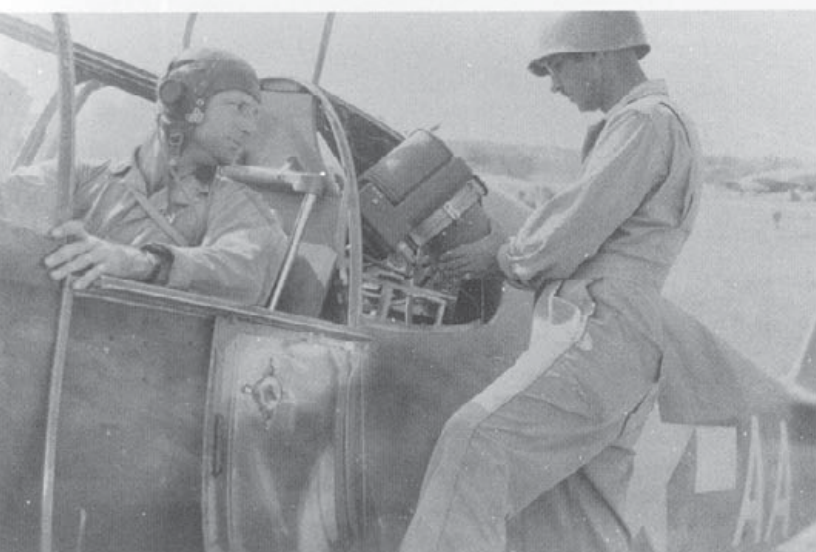
A mechanic adjusts the camera mounted behind the cockpit of a 111th TRS P-51 during 1944. By this time, the P-51 had been re-designated as the F-6 by the Army Air Corps. (James V. Crow)
