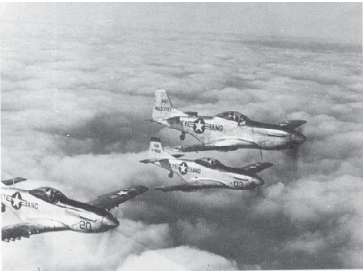
Several changes were made to these 165th Fighter Bomber Squadron/Kentucky ANG F-51Ds, including a fixed, non-retractable tail wheel, which was retrofitted to many Mustangs during the early 1950s. (ANG/HO)
