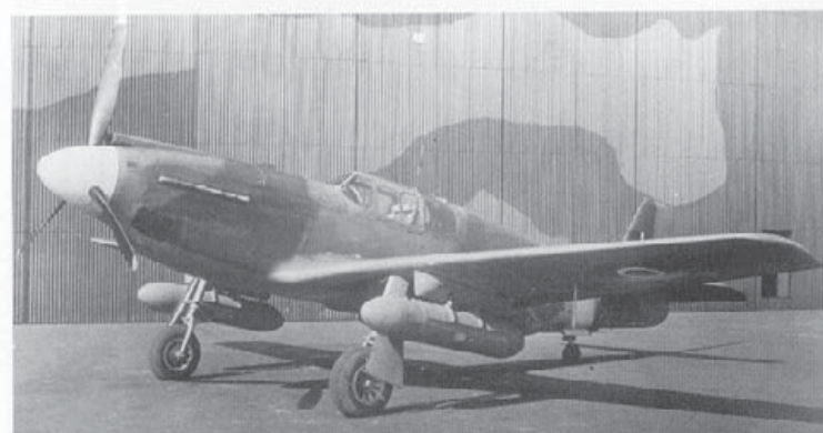
This Mustang I (AM 106) was used by the RAF at Boscombe Down for the flight testing of underwing drop tanks, bombs and large caliber cannons used for tank busting. (Imperial War Museum via R.L. Ward)
