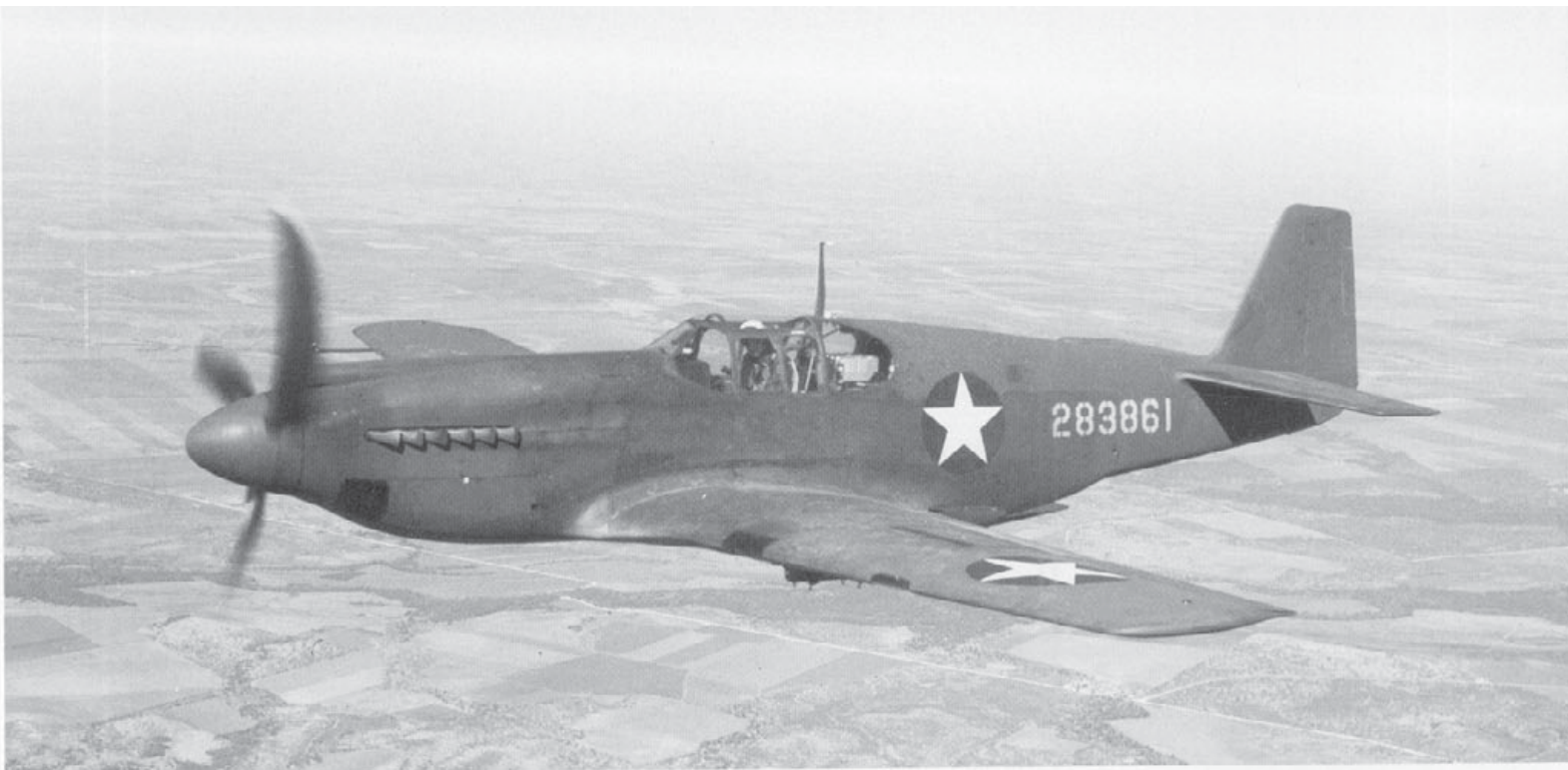
The A-36A Invader was a P-51 with upper and lower wing dive brakes and reinforced underwing pylons to carry 500 pound bombs. The A-36A was developed for use as a dive bomber and close support aircraft. (NAA)
