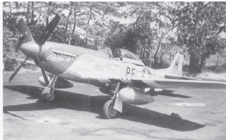
Patty IV , was a P-51D flown by Lieutenant Lawrence McCarthy while assigned to the 328th Fighter Squadron. The aircraft is equipped with a pair of 75 gallon metal drop tanks under the wings. Lieutenant McCarthy scored two and a half victories. (Keith Melville)
