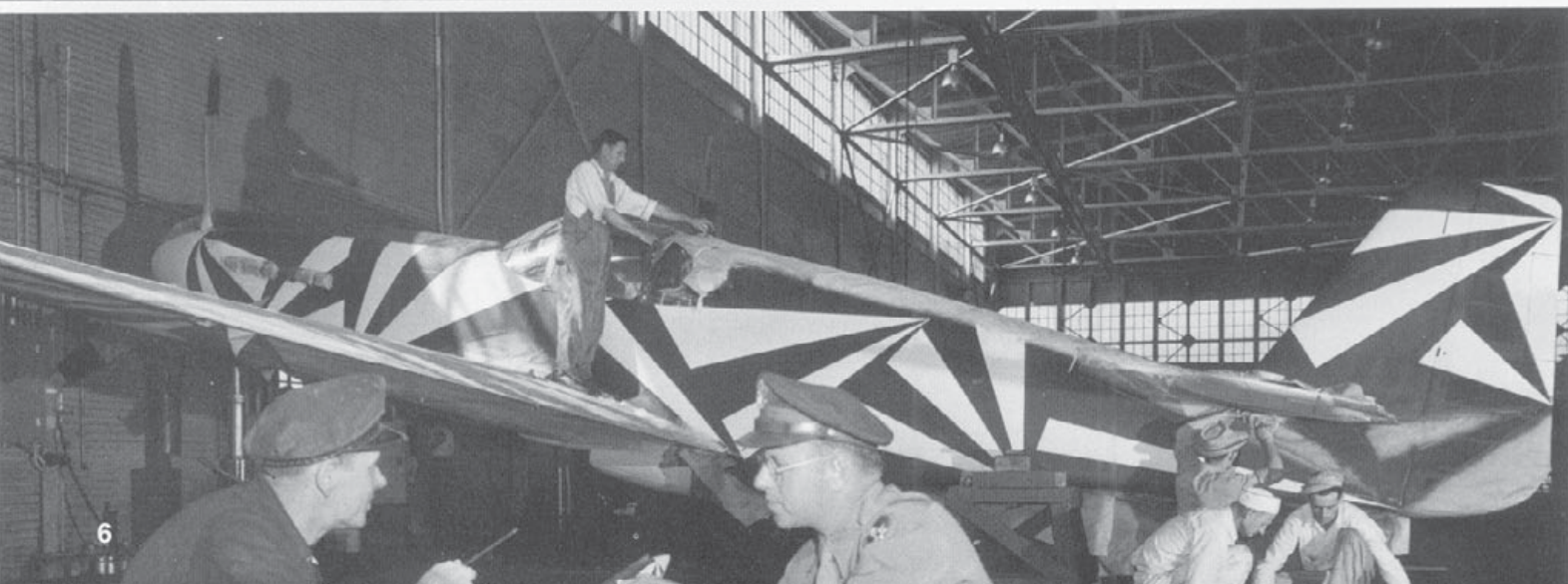
Captain Paul Hexter (center) designed the disruptive Black and White "dazzle" camouflage pattern being sprayed on this P-51 Mustang. The pattern was applied to the fuselage sides and the undersides of the wings and tail surfaces only. (USAAF)
