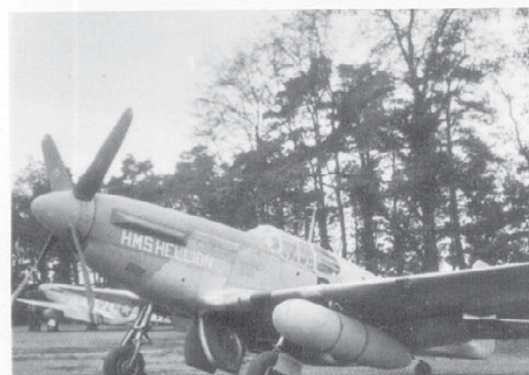
HMS Hellion was flown by Lieutenant Don Whinnem when he was assigned to the 486th Fighter Squadron at Bodney. The aircraft was equipped with two 110 gallon pressed paper underwing drop tanks. (Ernie McDowell)
