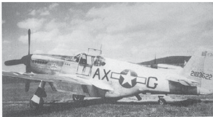
Satan's Son was an F-6C assigned to the 107th TRS at Middle Wallop during 1944. The F-6C had a camera in the left rear cockpit window, and another under the fuselage in front of the tail wheel. (Paul Miller via Merle Olmsted)
