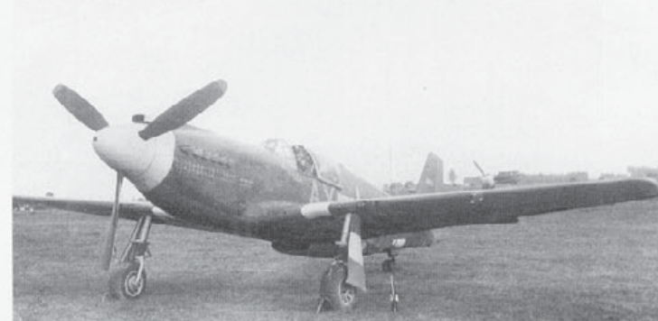
Jeanie , an F-6A from the 107th TRS on the ramp at Le Molay Airdrome, France, during the Summer of 1944. The aircraft had thirty-two mission markings on the nose in White and was equipped with a Malcolm bubble canopy, which could be and was fitted to many early Mustang variants. (Fred LePage)
