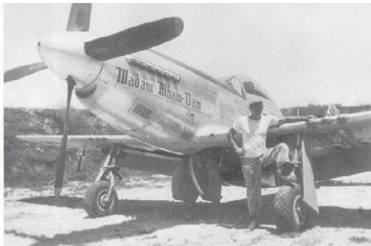
Madam Wham Dam , a 458th Fighter Squadron P-51D, parked in its revetment at North Field on Iwo Jima during 1945. The gun ports were taped over to retard dirt and corrosion in the gun barrels. (Ron Witt)
