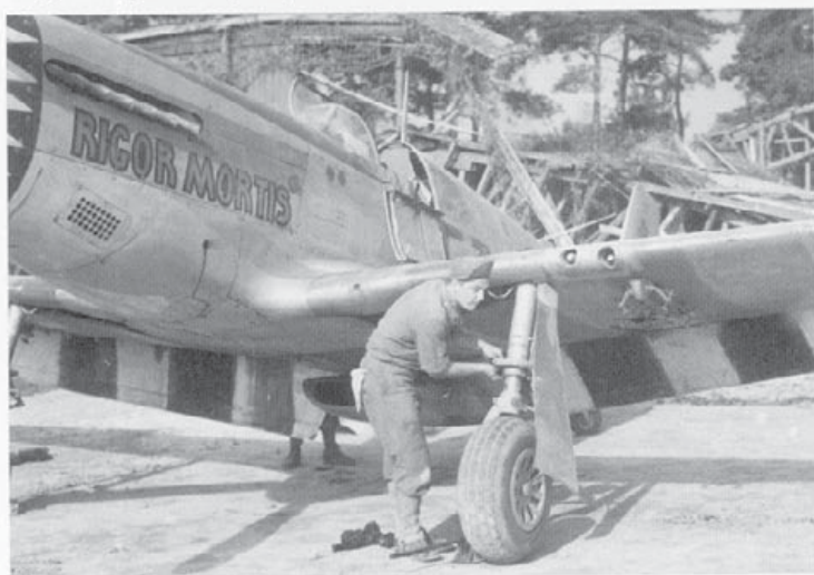
S/SGT Harold Staugler adjusts the landing gear oleo assembly on Rigor Mortis , a P-51C with the 353rd Fighter Squadron during September of 1944. (via Jeff Ethell)
