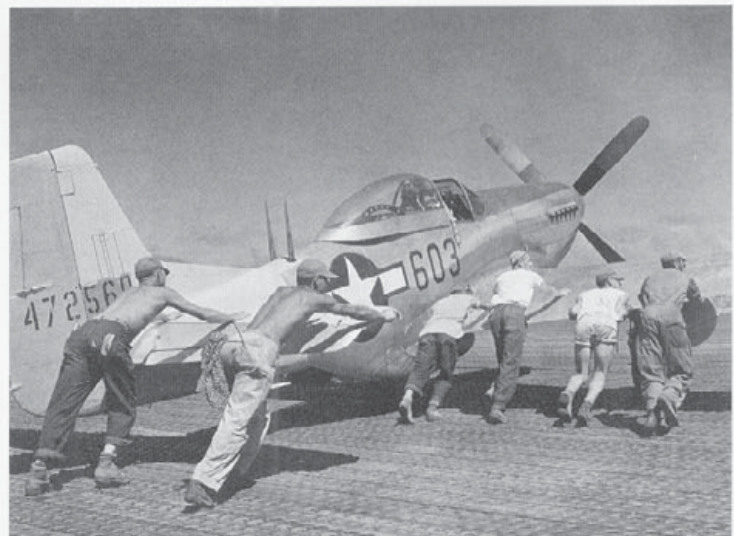
Ground crew personnel push a Yellow-tailed P-51D from the 462nd Fighter Squadron to its revetment at North Field on Iwo Jima during 1945. The antenna on the vertical fin was a tail warning radar. (USAAF)
